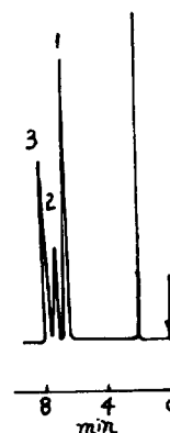
Fig. 5. Chromatogram of nitrochlorobenzene isomers on the PSCP-3-15-C5 column (10 m×0.25 mm) at 150°C; peaks: 1, m -nitrochlorobenzene; 2, p -nitrochlorobenzene; 3, o -nitrochlorobenzene.
